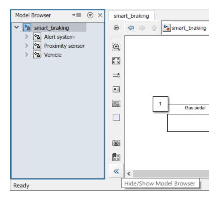
The Model Browser shows that all subsystems you view at the top level have subsystems of their own. Expand each subsystem node to see the subsystems it contains. You can navigate through the hierarchy in the Model Browser. For example, expand the Proximity sensor node and then select the Sensor model subsystem.
