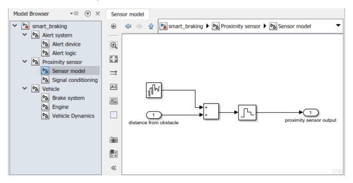
The address bar shows which subsystem you are viewing. To open the subsystem in a separate window, right-click the subsystem and select **Open In New Window**.
