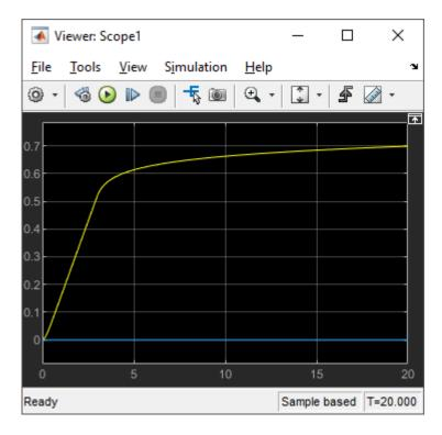
The first scope shows that the speed rapidly starts decreasing when the power is cut at time 3. The speed then asymptotically approaches zero but does not quite reach it. This is a limitation of modeling; dynamics at low speeds without external force requires a more complex representation. For the objective here, however, it is possible to make approximations. Zoom in on the position signal.
