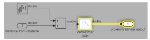
The Zero-Order Hold block in the Sensor model subsystem coverts the signal from continuous to discrete.
