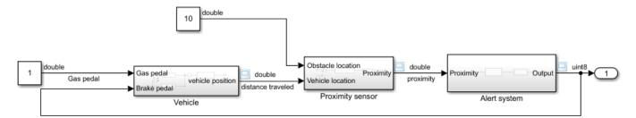
The model displays data types along the signal lines. Most signals are double, except the output of the Alert system. Double-click the subsystem to investigate.
