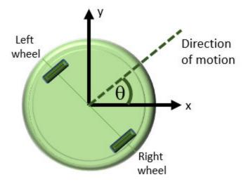
Each type of motion starts from a resting state, that is, both rotational and linear speeds are zero. With these assumptions, the linear and rotational motion components can be modeled separately.
