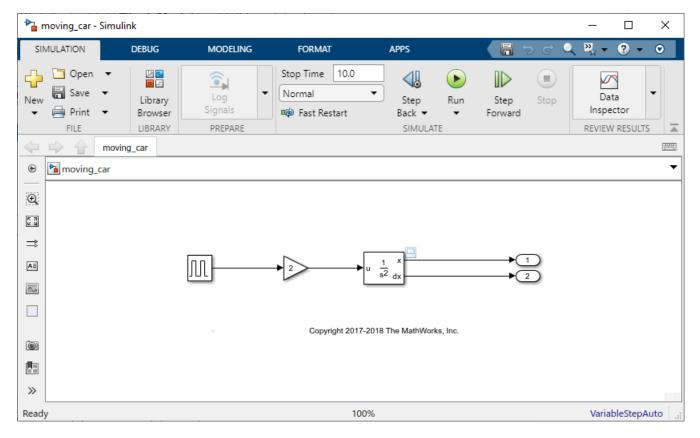
Simulating this model integrates a brief pulse twice to get a ramp. The results display in a Scope window. The input pulse represents a press of the gas pedal -1 when the pedal is pressed and 0 when it is not. The output ramp is the increasing distance from the starting point.
