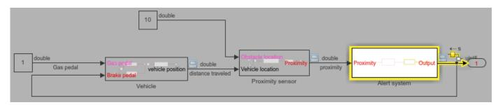
**3** To continue tracing the signal to its source, press the left arrow key.
