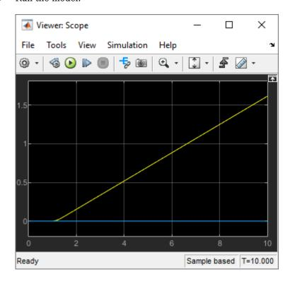
In this figure, the yellow line is the X direction and the blue line is the Y direction. Since the angle is zero and is not changing, the vehicle moves only in the X direction, as expected.
