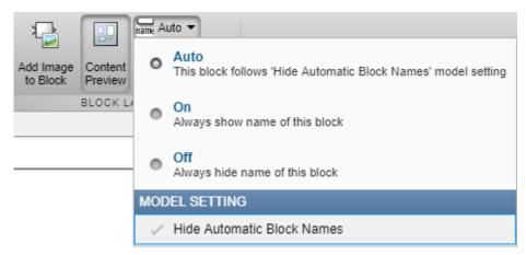
Arrange and rename the Subsystem blocks as shown. To change block names, double-click the block name and edit the text.
