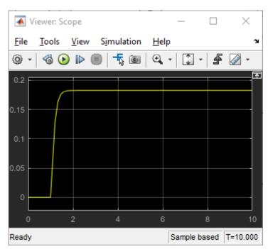
The simulation result exhibits the general expected behavior. There is no motion until force is applied at step time. When force is applied, the speed starts increasing and then settles at a constant when the applied force and the drag force reach an equilibrium. In addition to validation, this simulation also gives information on the maximum speed of the wheel for the given force.
