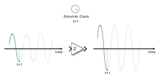
At each time step, each block computes its outputs from its inputs. Once all of the signals in a diagram are computed at a given time step, Simulink determines the next time step (based on the model configuration and numerical solver algorithms) and advances the simulation clock. Then each block computes their output for this new time step.
