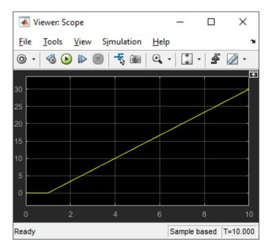
This simulation shows that the angle increases steadily when the wheels are turning with the same speed in opposite directions. You can make some model improvements to make it easier to interpret the angle output, for example:
